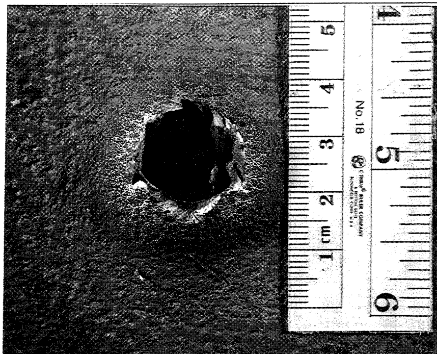
Figure 6. Photograph of typical exit hole in RHA.
