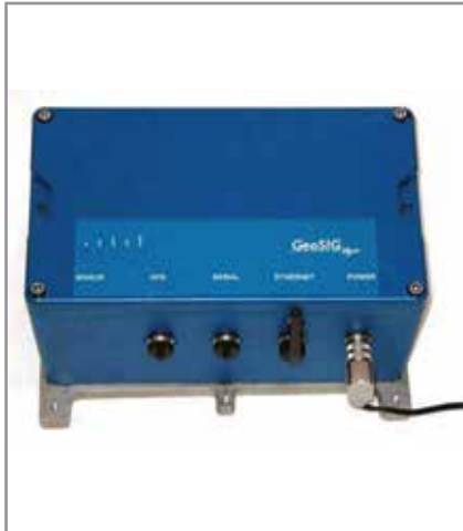
Figure 2. Left. The USGS NetQuake sensor (U.S. Geological Survey). Right. The USB version of the Quake-Catcher Network micro-electro-mechanical systems (MEMS) accelerometer (Courtesy of Stanford University: http://stanford.qcn.edu ).
