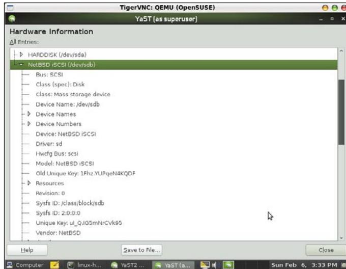
**Figure 5.** Let's see the properties for the attached device. We have it as a usual block device under the name of *sdX*
